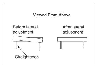
Figure 73. Before and after lateral wheel alignment (viewed from above).
